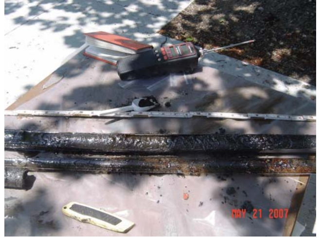
Photo #8 KSF-SB-17 (12-16') Coal tar saturated silty sand & gravel
