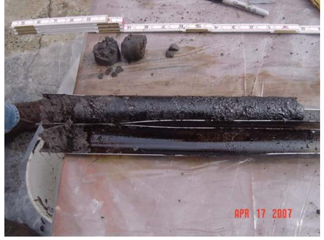
Photo#2 KSF-SB-01, (16-20') Coal Tar saturated sand and gravel overlying peat and clay
