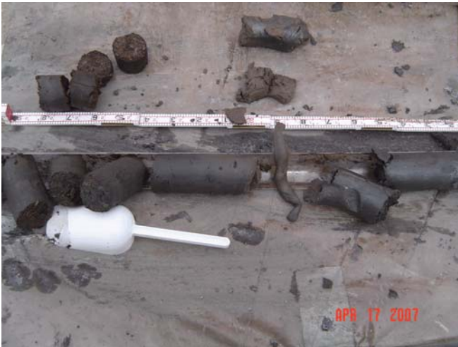
Photo#3 KSF-SB-04,(20-24') Clay layer (right) overlying clay and peat layer(left)
