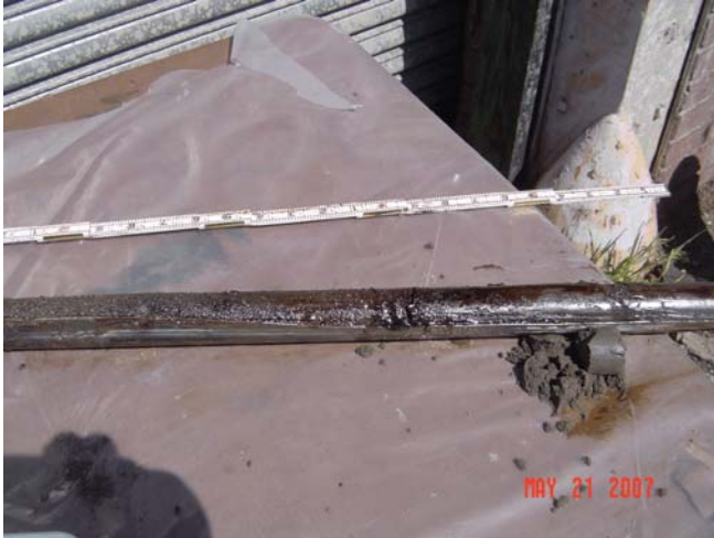
Photo#7 KSF-SB-14 (16-20') Coal tar saturated silty sand & gravel, clay layer 18.5-19.5'
