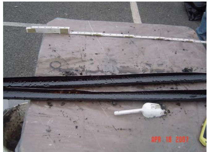
Photo#6 KSF-SB-09 (24-27.5') No recovery, coal tar coated sample tube
