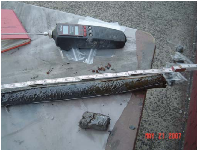
Photo#9 KSF-SB-22 (8-12') Coal tar saturated silty sand & gravel from 9' to 11.5'
